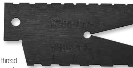
In use, the angle on the thread cutting tool is checked on the large precision-ground V at the end of the gage. The tool is then ground on the end to the width of the slot of whatever pitch is being turned. It is then set in the lathe using the half angle.
